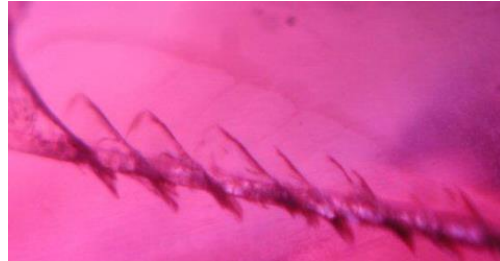
Bohemite needle with "satellite" secondary feathers in unheated ruby from Mogok
