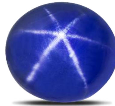
star sapphire: the inclusions are arranged according to a geometrical pattern, giving rise to bright lines
