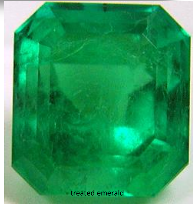
Surface reaching fractures in emeralds can be filled with artificial resins, wax, and epoxy polymers.
